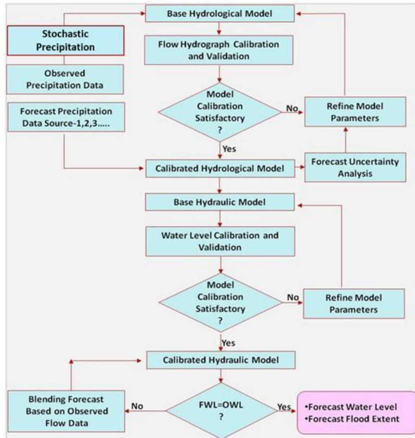
Figure 40: Flood forecasting model/components of HEC-RTS
