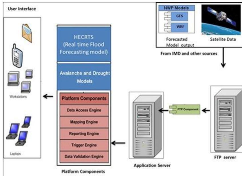
Figure 43: High level design of IOFS DSS
