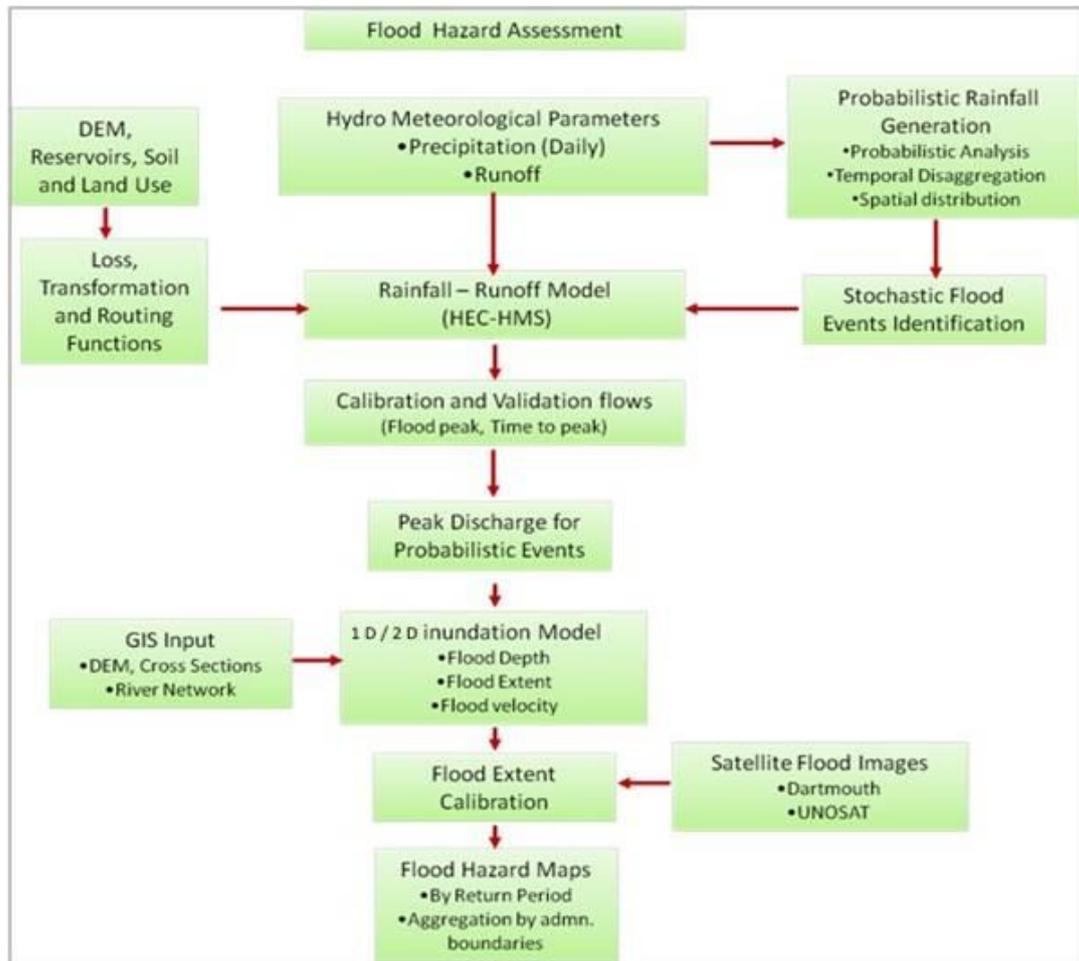
Figure 3: Flood hazard assessment framework
