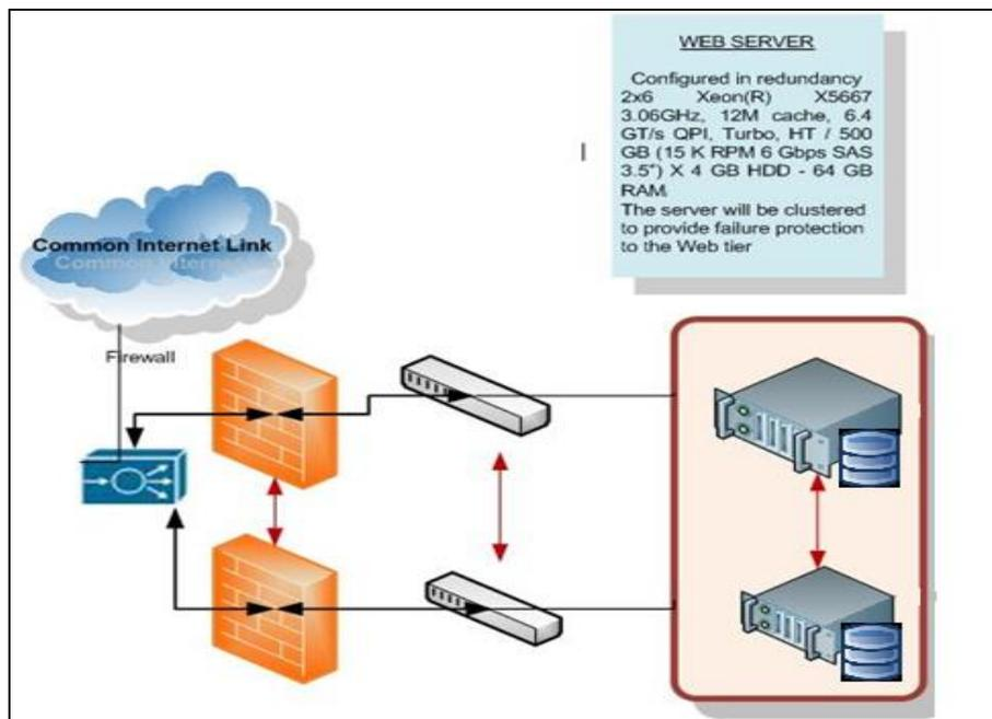
Figure 36: System Architecture
