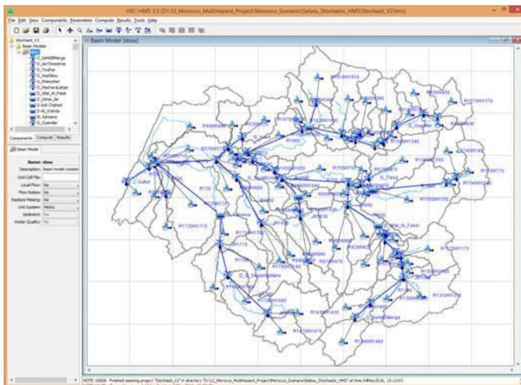
*Figure 6: HEC-HMS Hydrological model developed for Sebou Basin in Morocco (shown as an example only)*
