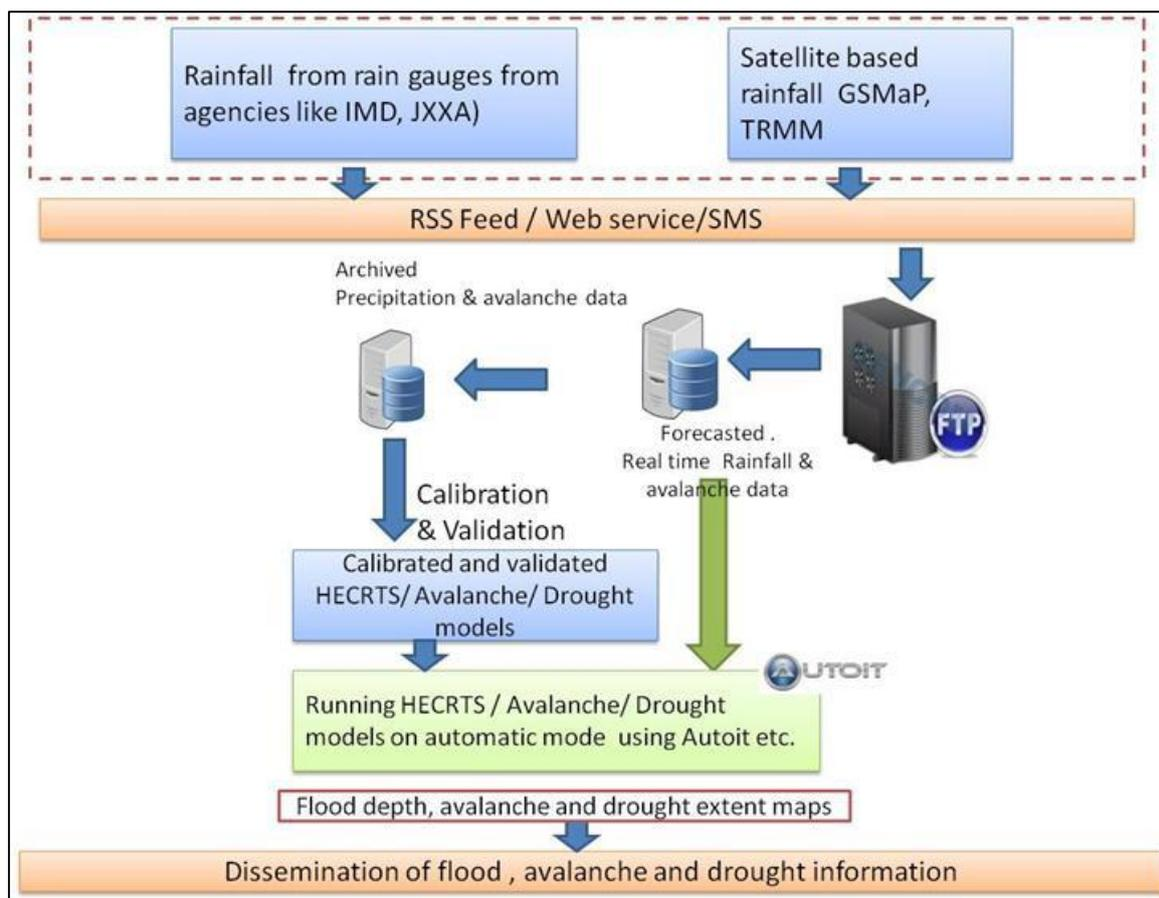
*Figure 44: Process flow of IOFS DSS dynamic analysis engine*
