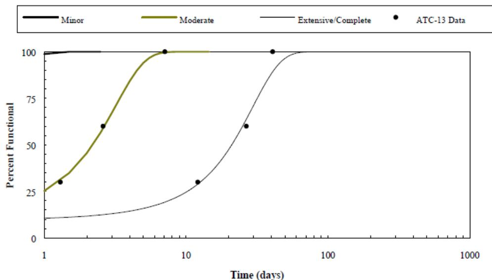
*Figure 24 Example Restoration Curves for Roads, after the HAZUS Multi-hazard Loss Estimation Methodology*
