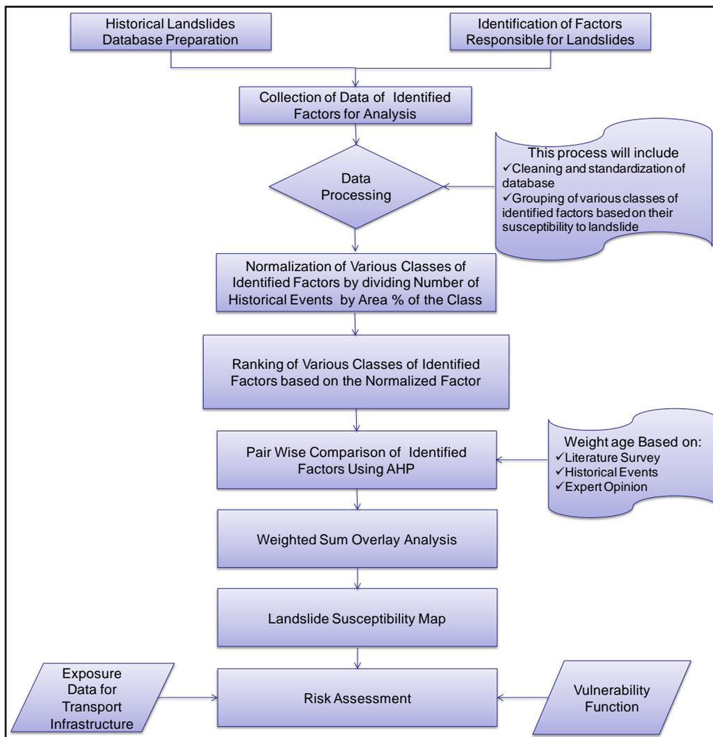
Figure 16: Overall approach for landslide susceptibility mapping
