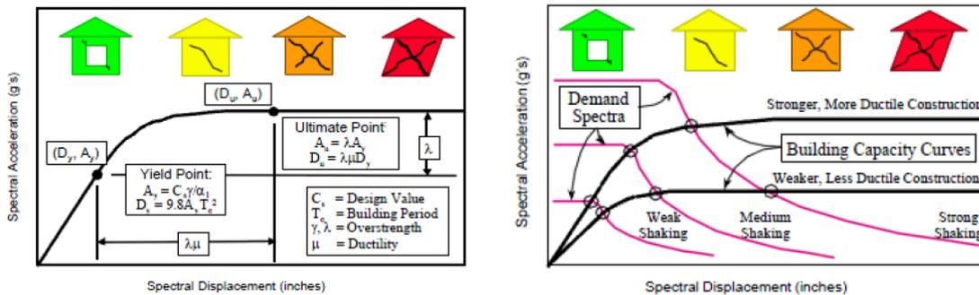
Figure 23 Illustration of the Capacity Spectrum Method: Example Capacity Curve (left) and Intersection of the Capacity Curves and Demand Spectra , after HAZUS Technical Manual
