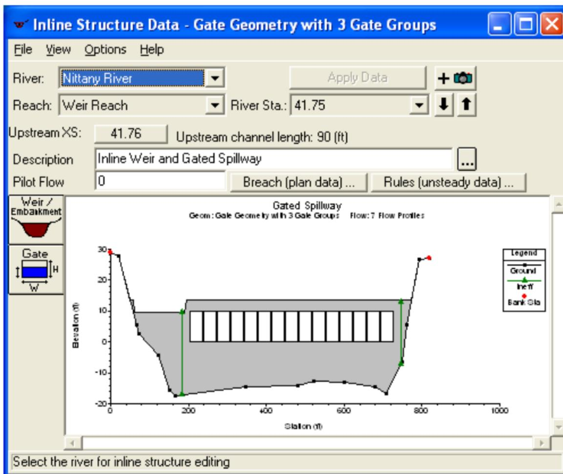
Figure 9: Typical incorporation of inline structures in hydraulic model
