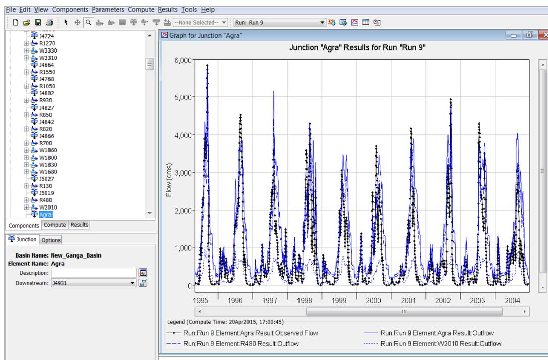
**Figure 7: Sample of typical calibration of gauge data**
