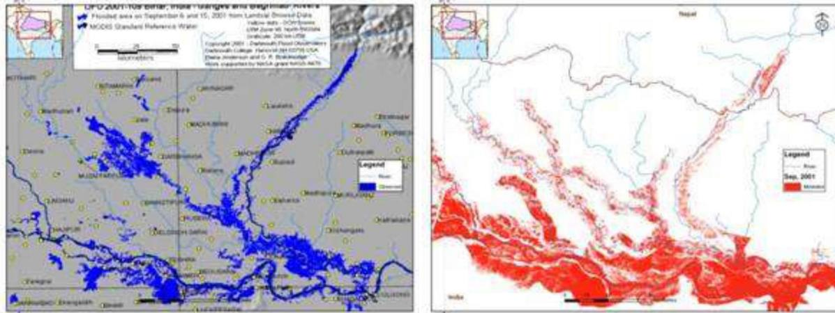
**Figure 10: Comparison between observed (left) and modeled (right) flood extents for an historical flood event**
