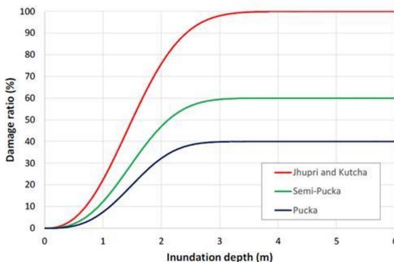
*Figure 21: A typical example of vulnerability curves for residential building types due to floods*
