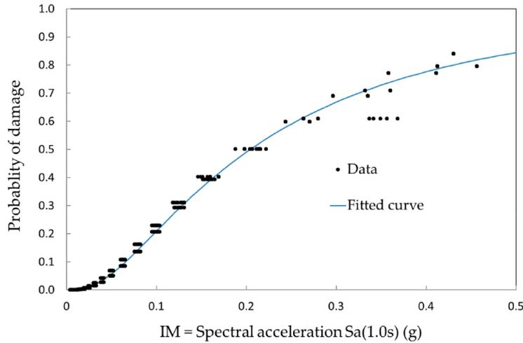
Figure 22 Example of the derivation of a vulnerability curve based on simulated damage data from scenario earthquakes, after Nollet et. al. (2018)<sup>30</sup>
