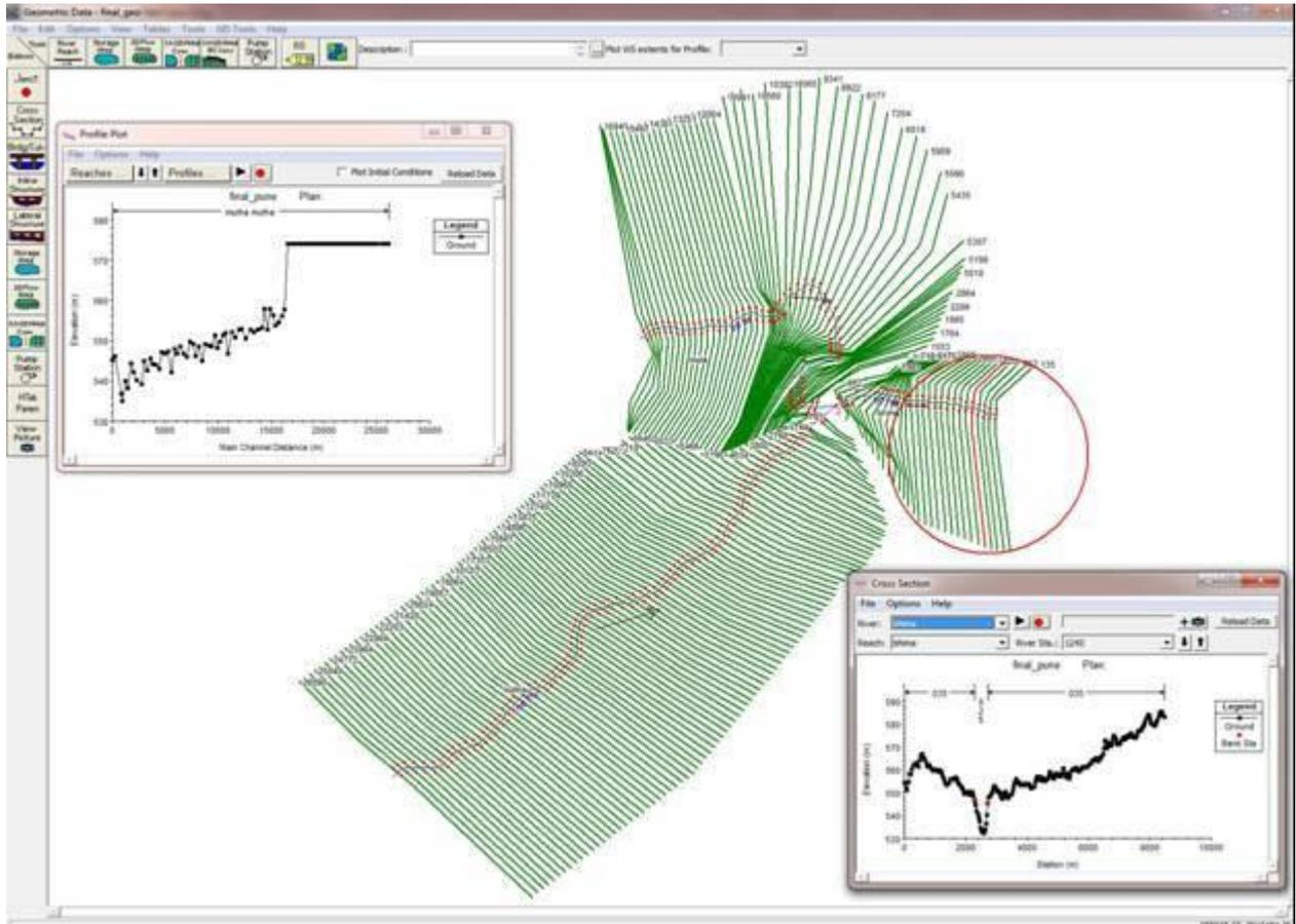
Figure 8: HEC-RAS geometry data for a sample basin
