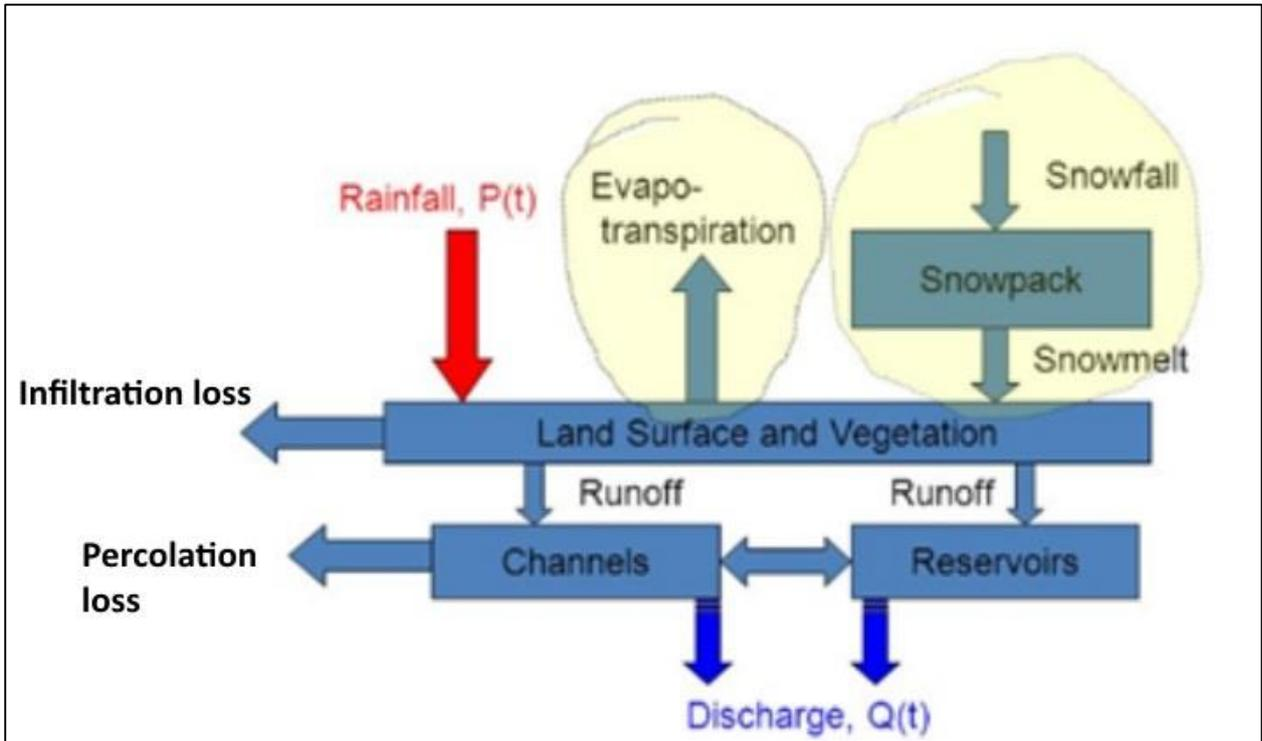
Figure 2: Flow diagram snow melt modeling in HEC-HMS
