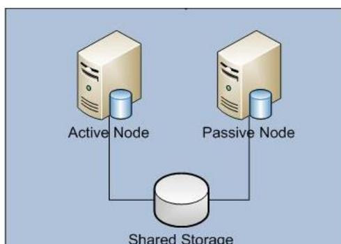
Figure 38: Redundant server
