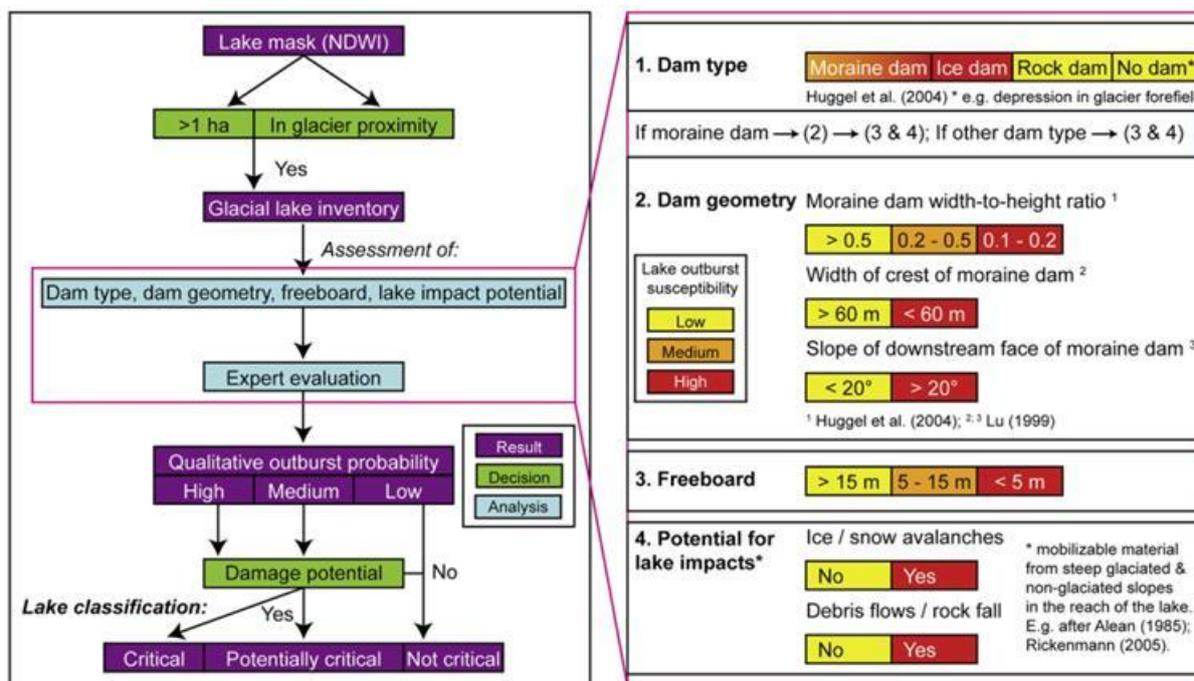
Figure 13: Methodology for Glacial Lake Inventory and Lake-Outburst probability assessment (Source: Worni, et.al, 2013).
