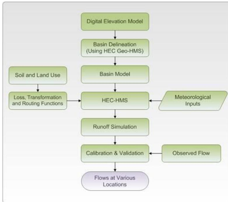
**Figure 5: Flowchart for hydrological modeling**
