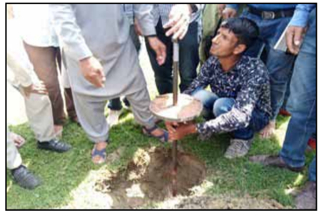
Figure 94 Practical session on use of hand penetrometer
