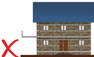
Large unsupported cantilevers
